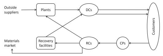
*Figure 3.* Product flows in the 3-stage network design problem of Özkır and Başlıgıl. *Key: CPs* — collection points, *DCs* — distribution centres, *RCs* — reverse centres.
